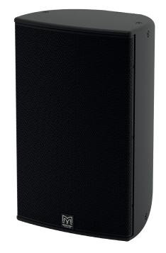
Ideal for medium-to-large rooms, the CDD15 is a very high-power, passive two-way system designed for installations that demand the ultimate in sonic performance from a single enclosure. It combines very high output capability with exceptional fidelity and coverage consistency. Its coaxial drive unit comprises a powerful 15" (380mm)/3" (75mm) voice coil LF driver and a 1.4" (35mm) exit HF compression driver with a 3" (75mm) pure titanium diaphragm.
