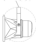
Single 13mmØ fixing point; suitable for M12 or 1/2" bolts.
