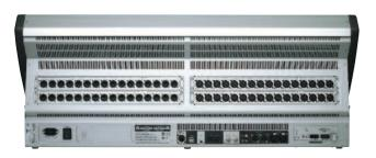
The Vi1 rear panel features 32 mic/line inputs, plus AES (4 channels) and SPDIF (2 channels) digital inputs. A Studer D21m system-based double card slot accommodates a range of I/O options including AES and MADI, which can be used to connect an optional Compact Stagebox or standard 64 channel Vi Series Stagebox, with all inputs and outputs fully patchable from the Vi1 control surface.
